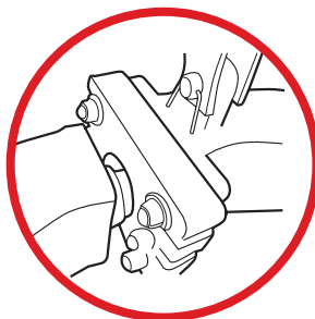
Blade arm centre bearing and boss replaced
