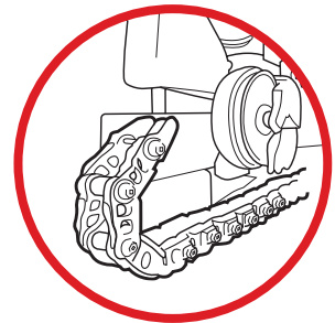
New track chains and guiding guards fitted
